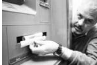
Cash is trapped by false withdrawal shutter
